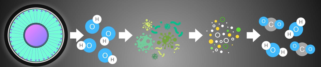
UV Light reacts with photocatalytic lining
