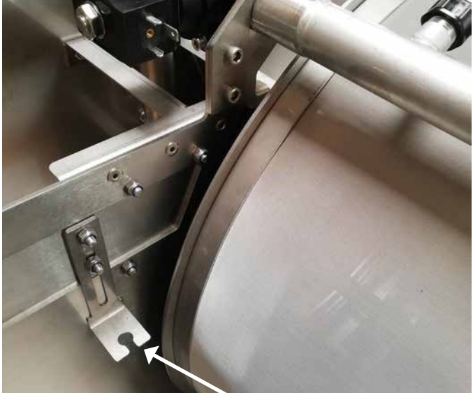
Filters without biochamber: Mount float switch here. Pure water area outside the drum
